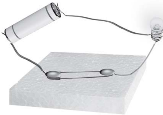
Fig. 14.7 An electric circuit
