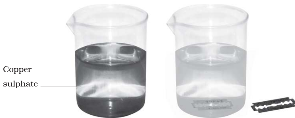
Fig. 6.4 Change in colour of the copper sulphate solution due to reaction with iron
