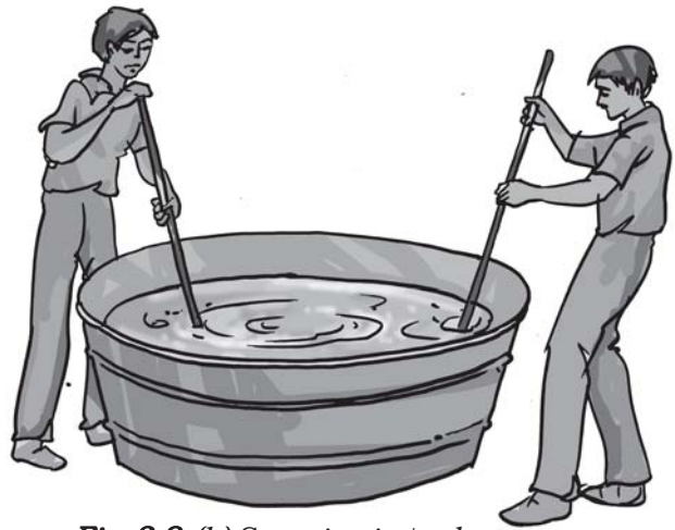
Fig. 3.8 (b) Scouring in tanks
