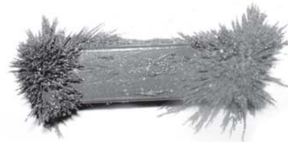
Fig. 13.7 Iron filings sticking to a bar magnet
