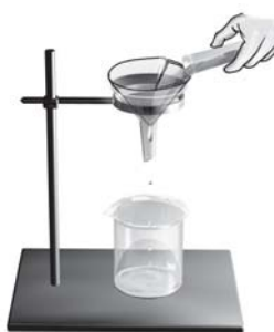
Fig. 5.10 Filtration using a filter paper
