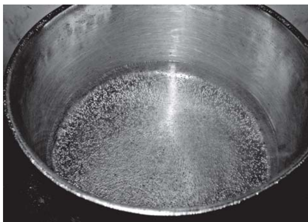
Fig. 15.10 Water contains air!
