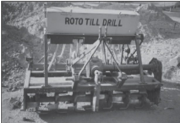
Fig. 5.12 : Roto Till Drill - A modern agricultural equipment
